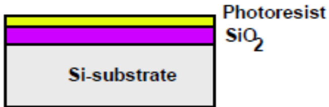
(b) After oxidation and deposition of negative photoresist
